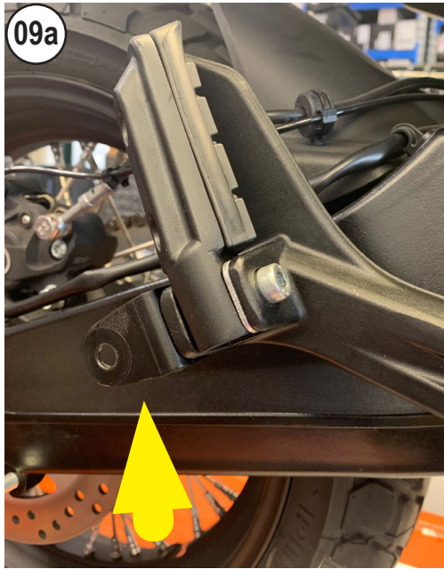
INSTALL THE BRACKET
