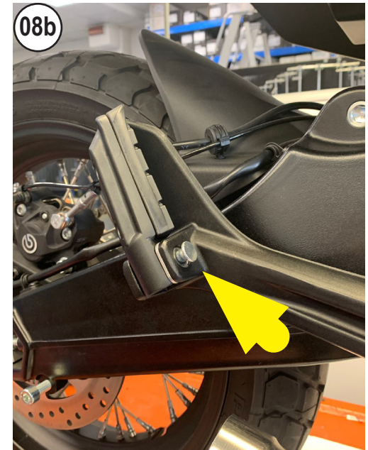
REMOVE THE SEEGER AND THE PIN
