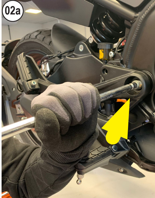
TAPPING THE PIN TO BRING IT BACK
