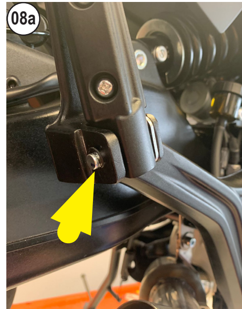
REMOVE THE SEEGER AND THE PIN
