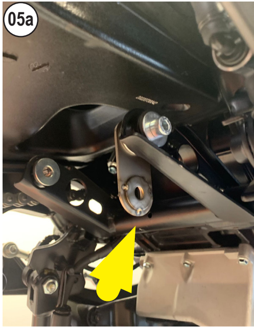
INSTALL THE BRACKET
