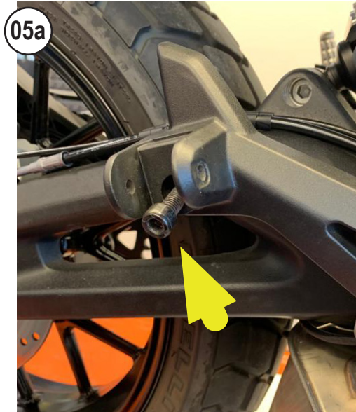
REMOVE THE SCREW AND THE FOOTPEG
