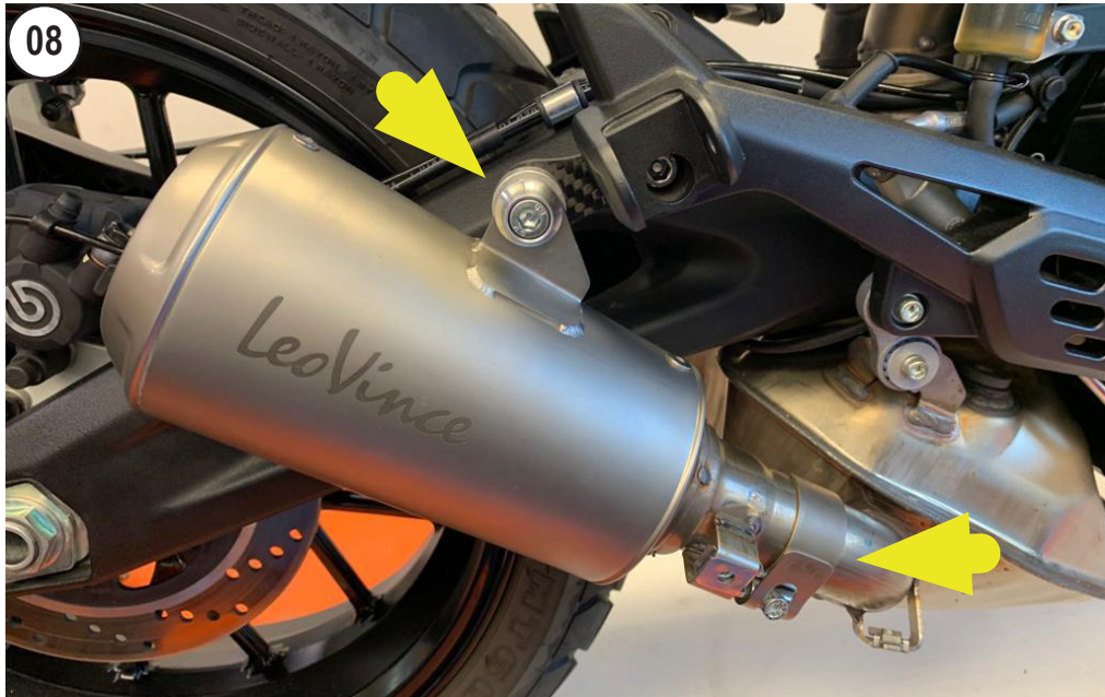
FIT THE CLAMP ON THE LeoVince MUFFLER AND INSTALL IT
