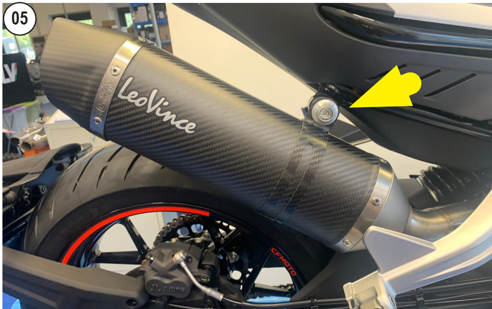
FIT THE CARBON CLAMP AND FASTENERS
