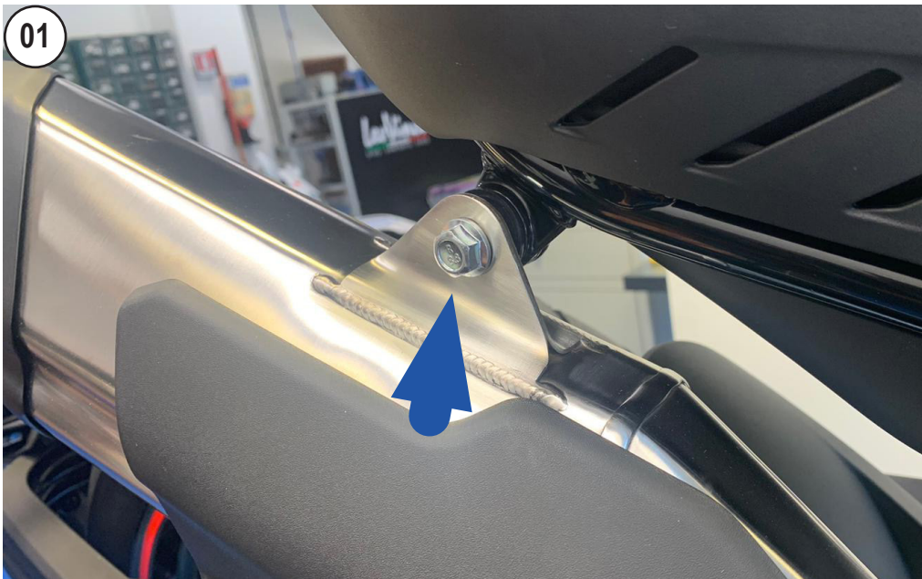
UNSCREW AND REMOVE THE STOCK MUFFLER
